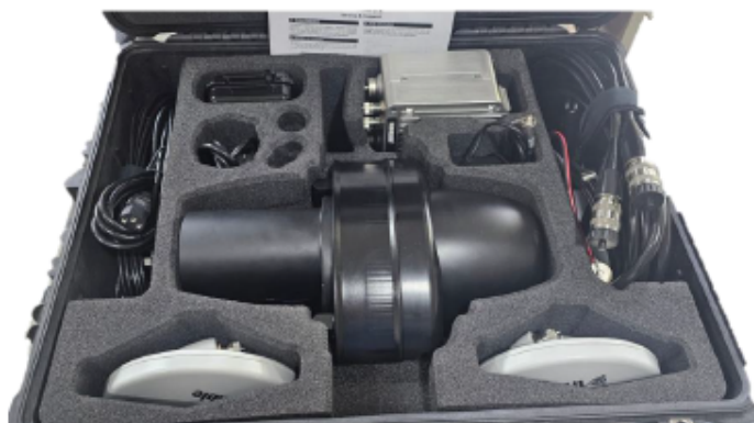
Figure 5: iWBMS integrated system
